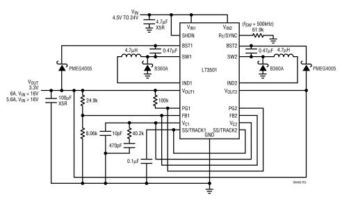
Figure 3. 4.5V to 24V  $_{IN},$  3.3V  $_{OUT}/6A$  Step-Down Converter
